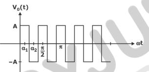
Above signal is modulated (have taken two switching per quarter cycle) keeping the odd half wave symmetry and odd nature of wave intact.
