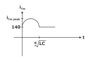
because t > 0 FD gets reverse biased and LC circuit current will also How through  $T_M$
