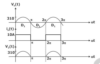
Average value of  $V_d(t) = \frac{1}{2\pi} \int_0^{\pi} 310 \sin \omega t \, d(\omega t) = \frac{310}{\pi} \text{ volt} = 98.67 \text{ volt}.$
