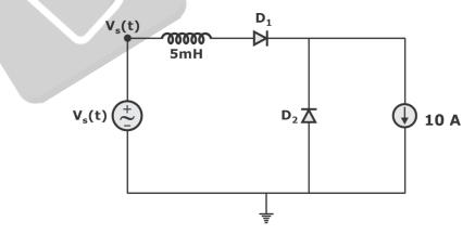
$0 \le \omega t \le \mu$  circuit is shown below
