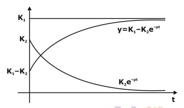
• We note that the responses to the systems have the same form, except for the constant terms  $K_1$  and  $K_2$ . It appears that the role of the numerator of the transfer function is to determine these constants, that is, the size of y(t), but its form is determined by the denominator.
