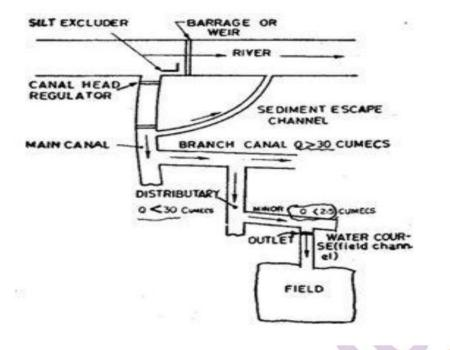
Applying the same reasoning, it can be established that the duty of water at the head of a minor will be less than that at the head of the watercourse; duty at the head of a distributary will be less than that at the head of a minor, duty at the head of a branch canal will be less than that at the head of a minor, duty at the head of the main canal will be less than the duty at the head of a branch canal will be less than the head of a branch canal.
