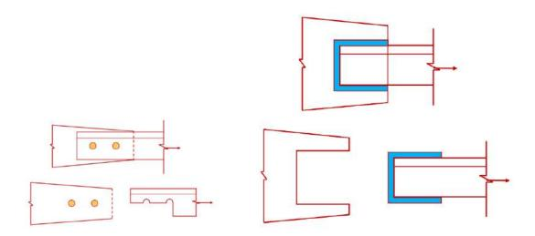
The strength of tension members is first determined under the various modes of failure, namely design strength due to gross section yielding ( $T_{dg}$ ), critical section rupture ( $T_{dn}$ ), and block shear strength ( $T_{db}$ ). The lowest of the three values listed above is the design strength of a member under axial tension ( $T_{d}$ ).
