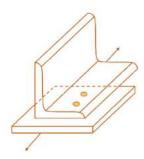
The shear lag effect can be reduced by using unequal angle sections with a longer leg connected and a shorter leg as an outstanding leg. To remove shear lag, the outstanding leg should also be connected. The shear lag effect is called the non-uniform stress distribution that occurs in tension members adjacent to a connection, in which all cross-section elements are not directly connected.
