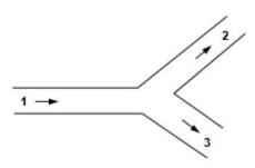
mass flow into the junction = mass flow out
