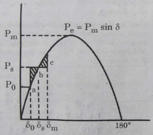
What is the condition of power at point 'b' if Pe is electromagnetic power and Ps is shaft power?
