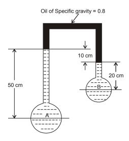
Determine the difference of pressures in the two pipes in terms of head of water and N/cm<sup>2</sup>, if the difference of liquid level in inverted U-tube be 10 cm. (15)
