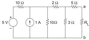
(b) Find current through  $5\Omega$  resistor in the circuit shown in Fig., using Thevenin's theorem. (10)
