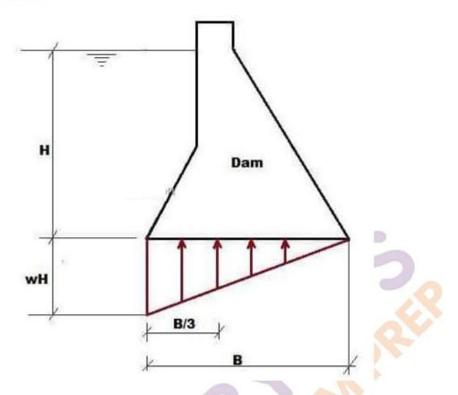
With reference to the figure, uplift pressure is given by
