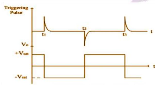
To change the bistable from one state to the other, the bistable circuit requires a suitable trigger pulse, and two such pulses are required for a full cycle. It is more commonly known as a "flip-flop" due to its actual operation, in which it flips into a logic state, remains there, then changes back to its original state.
