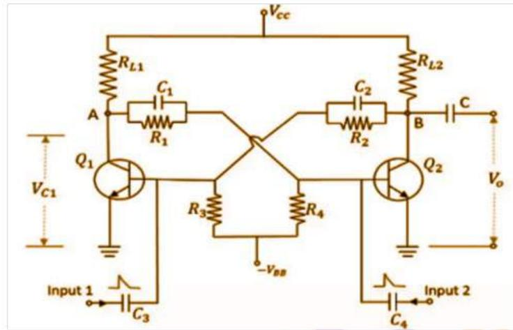
Using  $R_1$ , the output terminal of the first transistor is connected to the input terminal of the second transistor. In contrast,  $R_2$  connects the second transistor's output to the input of the first transistor. The resistances  $R_1$  and  $R_2$  are connected in parallel with two capacitors, also known as commutating capacitors, to improve the switching capability of the circuitry.
