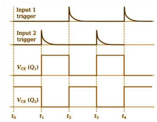
The output waveforms obtained at the terminal  $O_1$  and  $O_2$  are complementary to each other, always.
