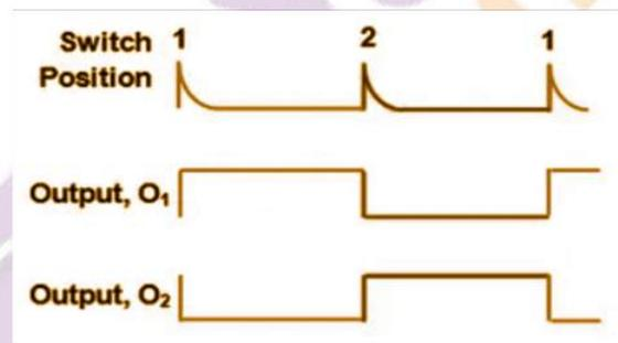
We can take the output from any of the two collector terminals. The only difference is the response we would get will be the inverse of the other collector terminal. We are getting a response with two stable states for two triggers.
