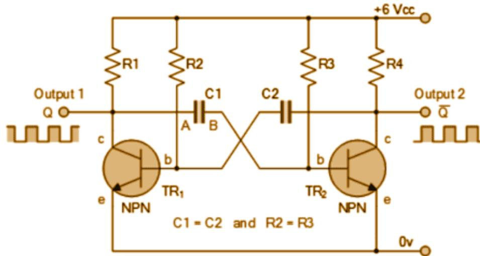
With this circuit, one stage conducts "fully-ON" (saturation). At the same time, the other is switched "fully-OFF"(cut-off), which creates an extremely high level of mutual amplification between the two transistors. The conductivity is transferred from one stage to another through the discharging action of a capacitor through a resistor.
