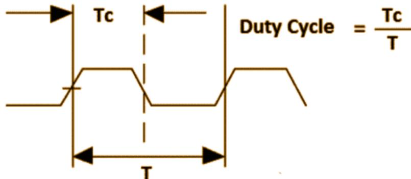
Based on this output rate, Duty Cycle =  $T_{ON}/(T_{OFF}+T_{ON})$  when the transistor has a collector output.
