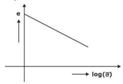
Base e = void ratio  $\overline{\circ}$  = effective stress
