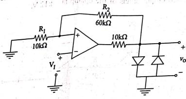
2. In the above circuit, if  $R_1$  is open circuit and  $R_2$  is short-circuit, redraw the characteristics.
