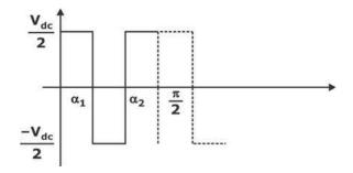
$$V_n = \frac{4\left(\frac{V_{dc}}{2}\right)}{n\pi} \ [1-2\cos\ n\alpha_1 + 2\cos n\,\alpha_2]$$
