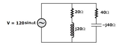
$$\begin{split} I_1 &= \frac{V}{Z_1} \\ I_1 &= \frac{120 \angle 0^{\circ}}{20 + j20} \\ |I_1| &= \frac{6}{\sqrt{2}} \\ (I_1)_{rms} &= \left(\frac{6}{\sqrt{2}}\right) \times \frac{1}{\sqrt{2}} = 3A \end{split}$$
