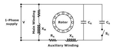
During steady state condition only main winding taking current.
