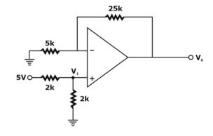
$$\Rightarrow V_1 = \left[\frac{5 \times 2}{2 + 2}\right] = \left(\frac{10}{4}\right) = 2.5 \text{ V}$$
