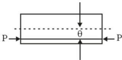
A tendon of rectangular pre-stress beam having cross-sectional area A is subjected to eccentric prestressing force P as shown in above fig. The stress at the top fiber is
