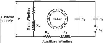
During steady state condition only main winding taking current. Hence, option D is correct.
