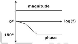
A. one LHP pole and one RHP zero at the same frequency.
