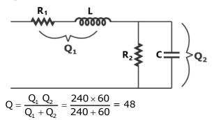
28. The network shown below has a resonant frequency of 150 kHz and bandwidth of 600 Hz. The Q-factor of the network is \_\_\_\_\_. (round off to nearest integer)
