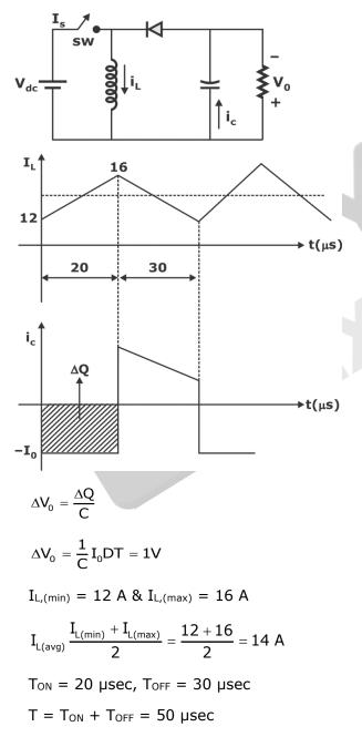
$$D = \frac{T_{ON}}{T_{ON} + T_{OFF}} = \frac{2}{5}$$
