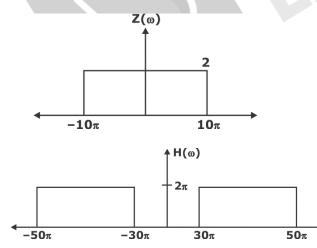
When input x(t) passes through the system h(t), the frequencies of  $42\pi$  and  $45\pi$  will pass through the band.
