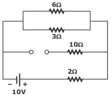
Voltage across 6  $\Omega$  is same as voltage across parallel combination of 6  $\Omega$  and 3  $\Omega.$
