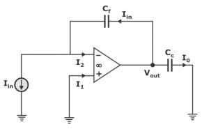
According to virtual ground,  $V_P = V_n = 0 V$
