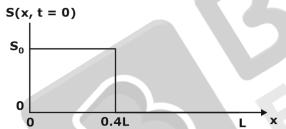
The boundary conditions of the problem are given by  $\frac{\partial s\left(x,t\right)}{\partial t}=0$  at the boundary point x=0 and x=L at all times. Consider D=0.1 m²/s.  $S_0=5$  µmol/m, and L=10, The steady concentration  $\tilde{S}\left(\frac{L}{2}\right)=S\left(\frac{L}{2},\infty\right)$  at the center  $x=\frac{L}{2}$  of the reservoir  $(in\mu/mol/m)$  \_\_\_\_\_. (in integer)
