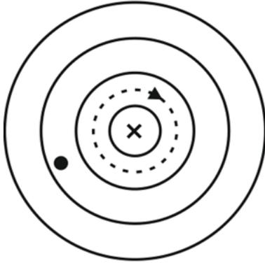
Make an amperian path as showing figure at r distance.
