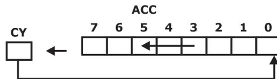
The least significant bit is set equal to the carry flag and the carry flag is set equal to the most significant bit.
