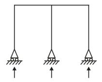
The above shown structure is unstable due to presence of reactions which are parallel.
