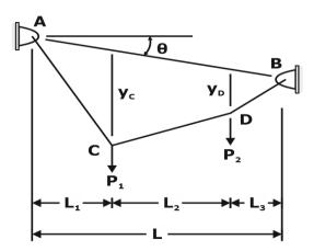
The tension at each member can be easily determined using the equation of equilibrium at each joint and the geometry of the structure.
