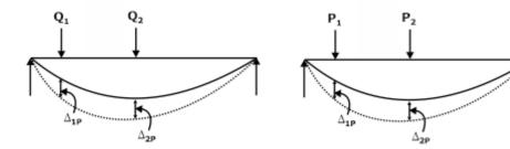
Virtual work done by P system of forces due to the displacements caused by Q system of forces =  $P_1\delta_{10}+P_2\delta_{20}$
