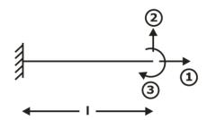
The cantilever beam shown in the figure above will be subjected to three displacements (1), (2) and (3).
