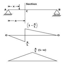
So, bending moment will be maximum if the load is at the section. For maximum negative shear force the load should be just to the left of section and for maximum positive shear force the load should be just right to the section.
