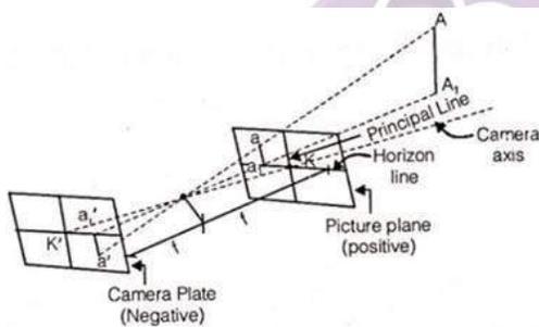
**(ii) Picture Plane:** A positive plane perpendicular to the camera axis.
