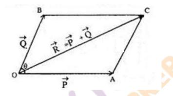
Let two vectors, P and Q operate on a particle O simultaneously. They are represented by the neighboring sides OA and OB of a parallelogram OACB formed from a point O in magnitude and direction. The diagonal OC running across O will thus indicate the size and direction of the consequent R.
