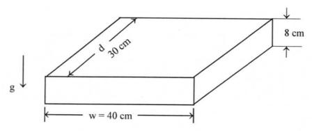
The top surface of the case has to dissipate 25W to the surrounding air, which is at 20°C. The emissivity of the surface is 0.6. Determine the temperature of the top surface, Given  $\beta$ =3.411×10<sup>-3</sup>/K.
