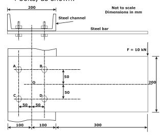
For an external load of 10 kN applied at the tip of the steel bar, the resultant shear load on the bolt at B, is \_\_\_\_\_ kN (round off to one decimal place).
