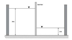
Taking the density of water as  $1000 \text{ kg/m}^3$ , and the acceleration due to gravity as  $10 \text{ m/s}^2$ . The maximum absolute bending moment
