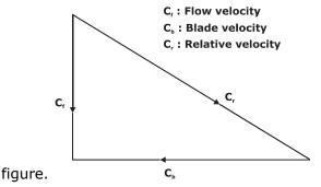
The diameter at this section is 3 m. The hub and tip diameters of the blade are 2 m and 4 m respectively. The water volume flow rate is  $100 \text{ m}^3/\text{s}$ . The rotational speed of the turbine is  $300 \text{ m}^3/\text{s}$ .
