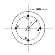
The rotor is driven by a motor at uniform angular speed of 10 rad/s. If one of the masses gets detached then the magnitude of the resultant unbalance force on the rotor is N (round off to 2 decimal places).
