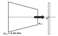
The inlet and outlet areas of the nozzle are  $0.1 \, \text{m}^2$  and  $0.02 \, \text{m}^2$ , respectively. Take air density as constant and equal to  $1.2 \, \text{kg/m}^2$ . If the inlet gauge pressure of air is  $0.36 \, \text{kPa}$ , the gauge pressure at point O on the plate is \_\_\_\_\_ kPa(round off to two decimal places).
