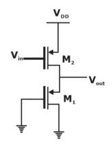
Ignoring the body effect, the ac small signal gain  $(\partial V_{out}/\partial V_{in})$  of the circuit is A.  $-g_{m2}(r_{01}||r_{02})$  B.  $-g_{m2}(1/g_{m1}||r_{01}||r_{02})$ C.  $-g_{m2}(1/g_{m1}||r_{02})$  D.  $-g_{m1}(1/g_{m2}||r_{01}||r_{02})$
