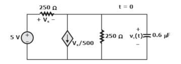
The time after which the voltage across the capacitor becomes zero (rounded off to three decimal places) is \_\_\_\_\_ ms.
