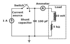
Initially, when the switch is open, the capacitor is discharged and the ammeter reads zero ampere. After the switch is closed, the ammeter reading keeps fluctuating for some time till it settles to a final steady value. The maximum ammeter reading that one will observe after the switch is closed (rounded of to two decimal places) is \_\_\_\_\_A
