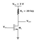
The channel length modulation coefficient is ignored. If the gate-to-source voltage  $V_{GS}$  is 1 V to keep the transistor at the edge of saturation, then the threshold voltage of the transistor (rounded off to one decimal place) is
