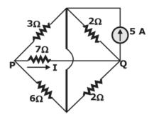
The current I flowing through the 7  $\Omega$  resistor between P and Q (rounded off to one decimal place) is \_\_\_\_\_A.
