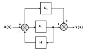
The transfer function  $\frac{Y(s)}{X(s)}$  of the system is
