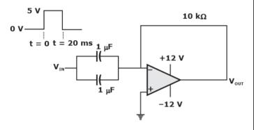
The output voltage  $V_{OUT}$  of this circuit at t = 0<sup>+</sup> (in integer) is \_\_\_\_\_ V.
