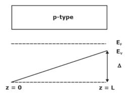
If the changes of an electron is q, then the magnitude of the electric filed developed inside this semiconductor bar is
