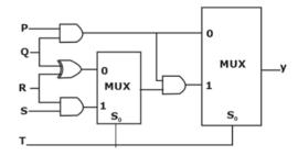
If all the inputs P, Q, R, S and T are applied simultaneously and held constant, the maximum propagation delay of the circuit is
