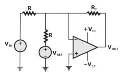
$\begin{array}{ll} \mbox{Assuming } |V_{IN}| \ll |V_{CC}| \mbox{ and } |V_{REF}| \ll |V_{CC}|, \\ \mbox{the condition at which } V_{OUT} \mbox{ equals to zero is} \\ \mbox{A. } V_{IN} = V_{REF} & \mbox{B. } V_{IN} = 2 + V_{REF} \\ \mbox{C. } V_{IN} = 0.5 \ V_{REF} & \mbox{D. } V_{IN} = 2 \ V_{REF} \\ \end{array}$
