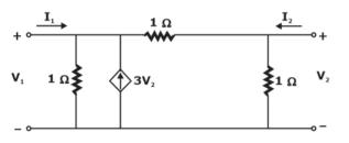
The admittance parameters, in Siemens, are A.  $y_{11} = 2$ .  $y_{12} = -4$ ,  $y_{21} = -4$ ,  $y_{22} = 2$
