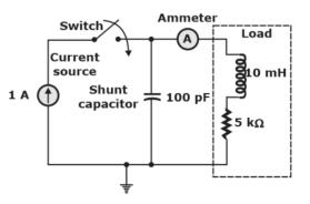
Initially, when the switch is open, the capacitor is discharged and the ammeter reads zero ampere. After the switch is closed, the ammeter reading keeps fluctuating for some time till it settles to a final steady value. The maximum ammeter reading that one will observe after the switch is closed (rounded of to two decimal places) is \_\_\_\_\_A
