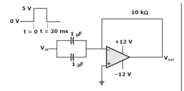
The output voltage  $V_{OUT}$  of this circuit at t = 0<sup>+</sup> (in integer) is \_\_\_\_\_ V.
