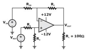
If  $V_{OUT} = 1$  volt for  $V_{IN} = 0.1$  volt and  $V_{OUT} = 6$ volt for  $V_{IN} = 1$  volt, where  $V_{OUT}$  is measured across  $R_L$  connected at the output of this OPAMP, the value of  $R_F/R_{IN}$  is
