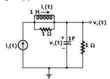
Current  $i_{L}(t)$  in the inductor and voltage  $v_{c}(t)$  across the capacitor are taken as the state variables, both assumed to be initially equal to zero, i.e.,  $i_{L}(0) = 0$  and  $v_{0}(0) = 0$  The system is
