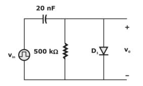
The difference between the maximum voltage and minimum voltage of the output waveform  $v_0$  (in integer) is \_\_\_\_\_V.
