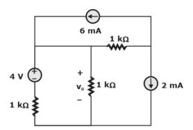
The value of  $v_0$  (rounded off to one decimal place) is \_\_\_\_\_ V.
