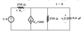
The time after which the voltage across the capacitor becomes zero (rounded off to three decimal places) is \_\_\_\_\_ ms.
