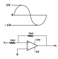
If the Op-amp is in positive feedback and the input voltage  $V_i$  is a sine wave of amplitude 1V,  $V_0 = ?$
