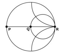
A. P : Open Circuit, Q : Short Circuit, R : Matched Load
