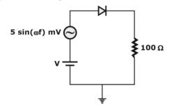
For  $\omega = 2 \times 10^6$  rad/s, the amplitude of the smallsignal component of diode current (in  $\mu$ A, correct to one decimal place) is \_\_\_\_\_.
