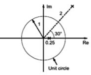
For the system to be stable, ROC should include the unit circle. From the given pole pattern, it is clear that to make the system stable, the ROC should be two-sided and hence the impulse response of the system should be also two-sided.
