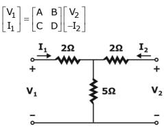
The parameter B for the given two-port network (in ohms, correct to two decimal places) is
