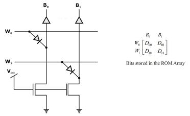
During the read operation, the selected word line goes high and the other word line is in a high impedance state. As per the implementation shown in the circuit diagram above, what are the bits corresponding to  $D_{if}$  (where i = 0 or 1 and j = 0 or 1) stored in the ROM?
