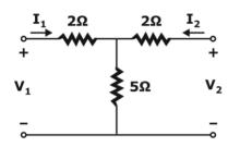
The parameter B for the given two-port network (in ohms, correct to two decimal places) is
