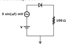
For  $\omega=2\times10^6$  rad/s, the amplitude of the small-signal component of diode current (in  $\mu A$ , correct to one decimal place) is \_\_\_\_\_.
