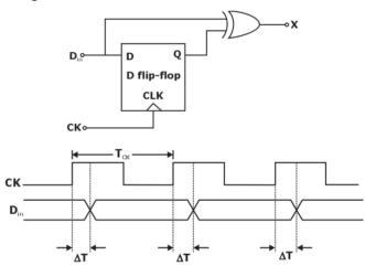
If the probability of input data ( $D_{in}$ ) bit transition in each clock period is 0.3, the average value (in volts, accurate to two decimal places) of the voltages at node X, is
