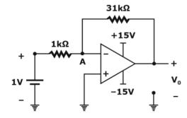
In the above circuit, assume the op-amp to be ideal. The voltage (in volts, correct to one decimal place) at node A, connected to the negative input of the op-amp as indicated in the figure is
