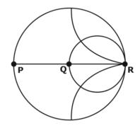
A. P: Open Circuit, Q: Short Circuit, R: Matched Load
