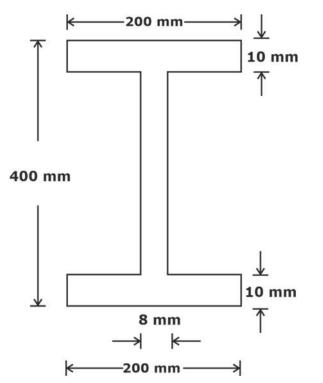
If the permissible stress is  $150 \text{ N/mm}^2$ , the bending moment M will be nearly.
