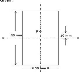
Load: P = 100 kN Eccentricity: e = 10 mm Width: b = 50 mm Depth: d = 80 mm
