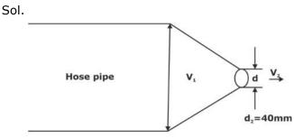
Flow rate:  $Q = 1200 \text{ Lpm} = 1.2 \text{ m}^3/\text{min}$ Force at joint will be given by:
