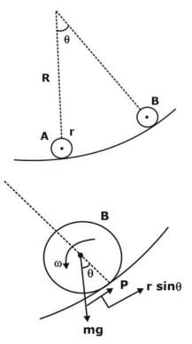
Disturbing force + Restoring force = 0 I $\alpha$  + mg rsin $\theta$  = 0 ------ (1)
