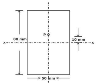
The maximum bending stress produced in the bar at xx is nearly \_\_\_\_\_\_.
