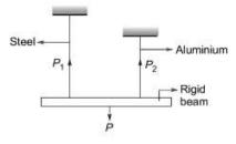
The rigid beam will remain in the center if and only if the elongation of both rods remains same.
