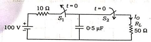
Before t = 0, switch  $S_2$  was OFF and switch  $S_1$  was ON for a long time. At t = 0,  $S_1$  is turned OFF and  $S_2$  is turned ON. Calculate the value of  $I_{\bar{O}}$  at t = 0.
