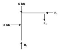
$\begin{array}{l} R_1 = 3 \ kN, \ R_3 - R_2 = 5 \\ (R_3 - 5) \ \times \ 15 - 3 \ \times \ 5 = 0 \\ R_3 = 6 \ kN, \ R_2 = 1 \ kN, \ R_1 = 3 \ kN \\ M_C = R_2 \ \times \ 15 = 1 \ \times \ 15 = 15 \ kN \text{-m} \end{array}$
