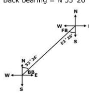
If the bearing is in quadrantal or reduced bearing system, in order to convert the fore bearing to back bearing it is only necessary to change the cardinal points by substituting N for S and E for W and vice versa. The numerical value of the bearing will remain the same.
