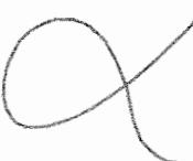
What is the ratio of vertical input signal frequency to that of horizontal input frequency ?
