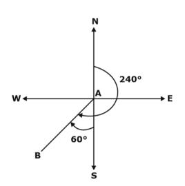
From figure, The reduced bearing is S60°W
