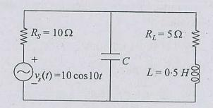
For the circuit as shown, what is the value of C that leads to maximum power transfer to the load, if the value of L is  $0.5 \, \text{H}$ ?
