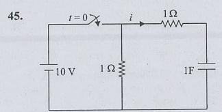
In the circuit as shown in figure, the switch is closed at t=0. The current through the capacitor will decrease exponentially with a time constant of magnitude
