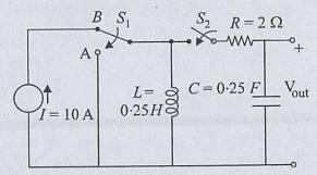
For the circuit as shown, consider that switch  $S_1$  has been in position B for a very long time and switch  $S_2$  has been open all the time. At time t=0, the switch  $S_1$  moves to position A and switch  $S_2$  closes instantaneously. What is the value of  $V_{\text{out}}$  at  $t=0^+$ , assuming initial charge on C=0?
