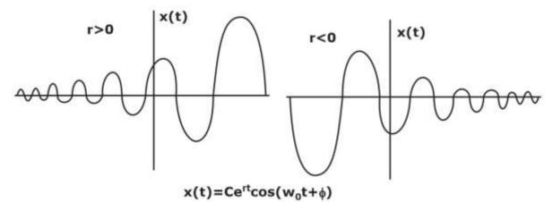
Sinusoidal signal multiplied by decaying exponential is refrred as damped exponential. Similarly for the discrete time characteristic where t becomes n.
