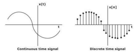
**Sampling:** Creation of discrete time signal from continuous time signal by defining successive samples of continuous time signal for a constant interval of time.
