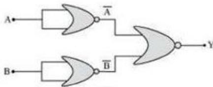
Identify the correct logic operations performed by the above circuit consisting NOR gates?
