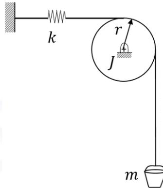
The pulley radius is  $r$  and its mass moment of inertia is  $J$ . Assume that the mass is vibrating harmonically about its static equilibrium position. The natural frequency of the system is
