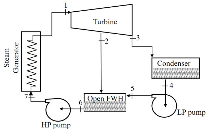
Specific enthalpy of steam at location 2 is  $2624 \text{ kJ/kg}$ , specific enthalpy of water at location 5 is  $226.7 \text{ kJ/kg}$  and specific enthalpy of saturated water at location 6 is  $708.6 \text{ kJ/kg}$ . If the mass flow rate of water entering the open feed water heater (at location 5) is  $100 \text{ kg/s}$  then the mass flow rate of steam at location 2 will be \_\_\_\_\_  $\text{kg/s}$  (round off to one decimal place).
