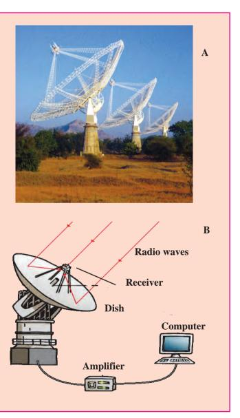
18.4 A. Radio telescope (photograph) B. The structure of a radio telescope
