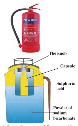
13.12 Internal structure of fire extinguisher
