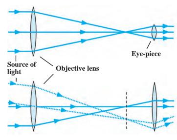
18.1 A refracting telescope
