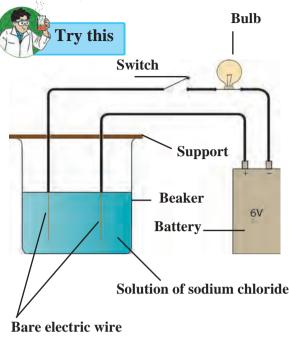
5.8 Testing the electrical conductivity of a solution
