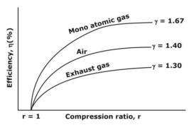
• Work Output  $W_{net} = W_{1\rightarrow 2} + W_{3\rightarrow 4} = \frac{P_1 V_1}{\gamma - 1} (r_P - 1) (r^{\gamma - 1} - 1)$
