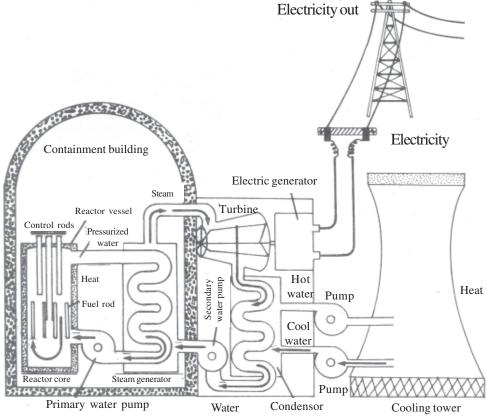
Fig. 28.8: Conversion of nuclear energy into electrical energy
