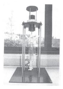
Fig. 31.5: Lab-scale batch OBR
