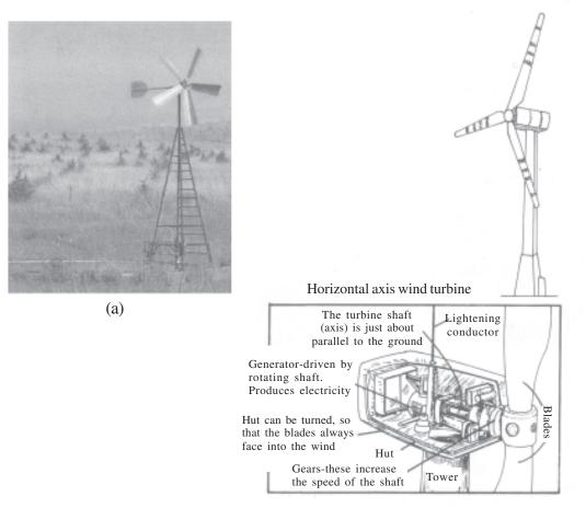
Fig. 29.4: (a) Wind mill used for pumping water (b) Wind mill used for generating electricity showing detail of shaft
