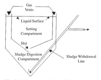
Fig. 31.4: Components of Imhoff tank
