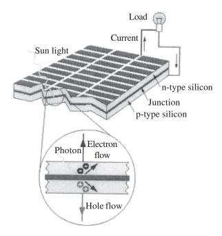
Fig. 29.3: Photovoltaic cell
