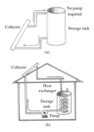
Fig. 29.2: Two active solar systems for heating water: (a) thermo siphon system.
