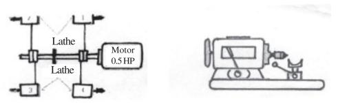
Fig 31.1 (a): Monoblock lathe (Q) consumes 80% less energy than conventional lathe (P)
