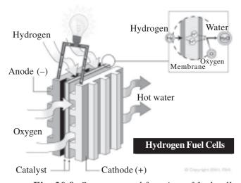
Fig. 30.8: Structure and function of fuel cell
