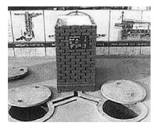
Fig. 25.1: Two pit pourflush toiled (Sulabh Shauchalaya)
