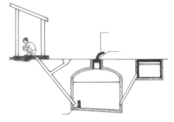
Fig. 18.6: Biogas digester
