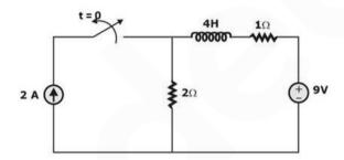
The switch is opened at t = 0. The energy stored in the inductor at steady state is.
