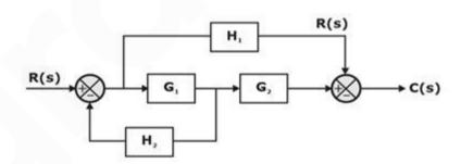
$$\text{A. } \frac{\text{G}_{1}\text{G}_{2}}{1+\text{G}_{1}\text{H}_{2}}$$
