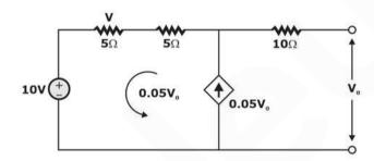
$$10 + 10 (0.05 V_0) - V_0 = 0$$
