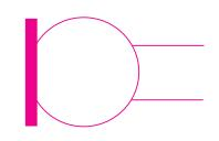
Fig. 18.9 Symbol of a microphone
