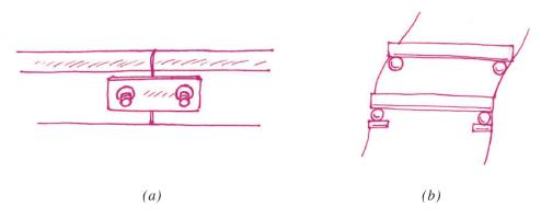
Fig. 14.12 (a) Gap in railway tracks (b) Girders in iron bridges placed on rollers
