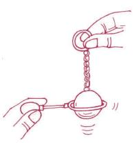
Fig. 14.5 Ball and ring experiment to demonstrate thermal expansion
