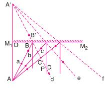
Fig. 15.5 Image formation by a plane mirror
