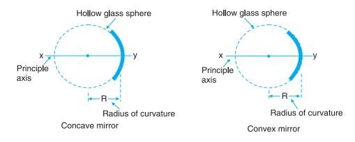
Fig. 15.11 Some important terms of spherical mirrors
