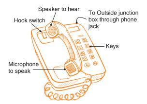
**Fig. 18.11 (a)** The basic structure of a wired phone set (In actual phone there is a provision so that your voice does not reach and disturb you)
