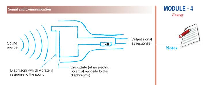
Fig. 18.10 (a) Structure of a condenser (capacitor) microphone
