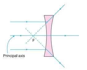
Fig. 15.24 Diverging action of a concave lens
