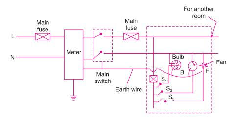
Fig. 17.18 Household circuit (one bulb, one fan and one plug point)
