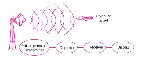
Fig. 18.8 A simple sketch of components of RADAR
