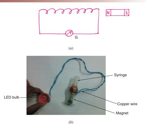
**Fig. 17.12** To understand the above principle better, we will try to make a simple experiment, Take a disposable syringe (the one with which a doctor administers injections). Make a 150 turns thin copper insulating wire at the middle of the syringe. Join the two ends of copper wire to Light Emitting Diode (LED) through connecting wire. LED may be fixed inside the plastic bottle capas in Fig. 17.12(b). Placed one cylindrical magnet
