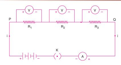
Fig. 16.7 Resistors in series
