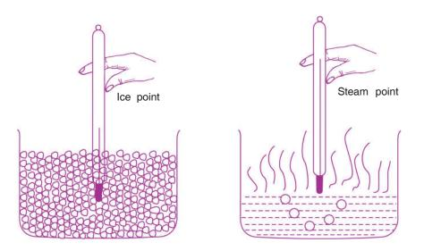
Fig. 14.2 Calibration of a thermometer
