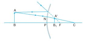
Fig. 15.15 Image formation by a convex mirror
