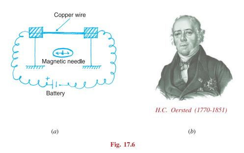
The principle of the magnetic effect of electric current used in many appliances like motor etc.
