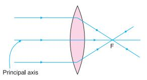
Fig. 15.23 Converging action of a convex lens
