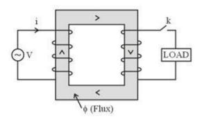
By the use of magnetic core, flux linking in between primary and secondary case to flow. Core at the transformer help to provide magnetic path by reducing the reluctance of the common magnetic circuit.
