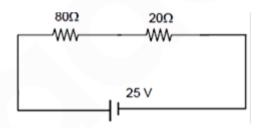
Voltage across 80 ohm resistance,  $V_{800hm} = 80/(80+20) \times 25 = 20 \text{ V}$
