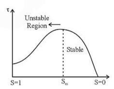
In the region in between the ship lies from S=1 to  $S=S_{mt}$ , the motor comes under the pull-out torque region or breakdown region. In this region the induction motor become unstable, where the slip is nearly equal to 1.
