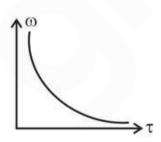
The given characteristic is the speed-torque characteristic of D.C. series motor.
