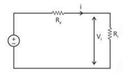
For the ideal voltage source, the total input voltage should be comes across the load resistance, which is only possible when there is no voltage drop across  $R_g$  i.e.,  $R_g$  should be equal to zero.
