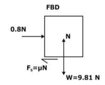
Normal reaction on the clock, N = mg
