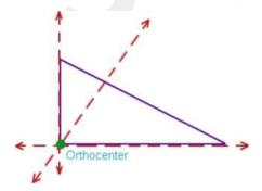
Orthocenter is the point of intersection of the altitudes. Each leg in a right triangle forms an altitude. So, in a right-angled triangle, the orthocenter lies at the vertex containing the right angle.
