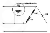
The load is connected across 3-phase, 400 V, 50 Hz supply with phase sequence abc. The reading of the wattmeter (in watts) is \_\_\_\_\_. (round off to integer value) Sol. The reading of the wattmeter is given asW = voltage across pressure coil x current through current coil x Cosine
