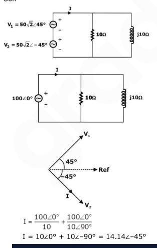
$\therefore$  Phase angle of current I with respect to voltage V1 in the circuit is  $-90^{\circ}.$
