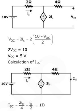
writing KVL in outer loop,  $10 - 2i_x - 4I_{SC} = 0$ By putting the value of  $i_x$  from equation (1)  $10 - 2 \times 2I_{SC} - 4I_{SC} = 0$
