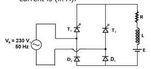
Sol. Given that firing advanced angle =  $140^{\circ}$ So, the firing angle =  $180^{\circ} - 140^{\circ} = 40^{\circ}$
