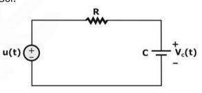
$$V_{c}(t) = V_{c}(\infty) + [V_{c}(0) - V_{c}(\infty)]e^{-t/\tau}$$
