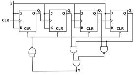
Then the modulus of the given counter is \_\_\_\_\_.(Assume  $Q_3$  be MSB &  $Q_0$  be LSB)
