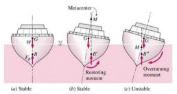
Moment due to weight and buoyant forces balance from overturning effect.
