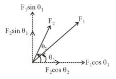
$\Sigma H = F_1 \cos \theta_1 + F_2 \cos \theta_2$   $\Sigma V = F_1 \sin \theta_1 + F_2 \sin \theta_2$ Resultant force =  $\sqrt{(\Sigma H)^2 + (\Sigma V)^2}$  $\tan \theta = \frac{\Sigma V}{\Sigma H}$
