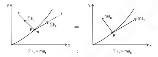
If the particle is moving in a curved path of radius of curvature  $\rho$  and having the velocity v at any instant,
